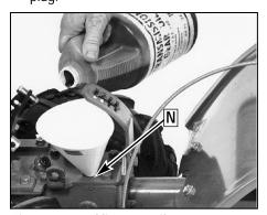
Figure 2-10: Adding gear oil.
